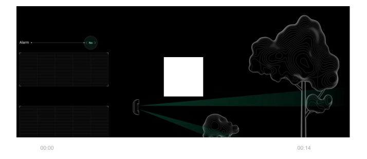
MotionCam Outdoor features two independent IR sensors, the signals of which are analyzed by a two-stage LISA algorithm. As soon as both IR sensors detect
